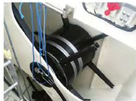
Left: the assembly order with a hull that is split vertically will be familiar to raceboat and multihull builders though still rare in superyachts; but there are big gains to be had in using more time to complete work inside the boat before the parts are joined. Above: like an FD's halyard take-up reel but bigger. Onto this 1.6m drum is wound nearly half-a-tonne of furling code zero
